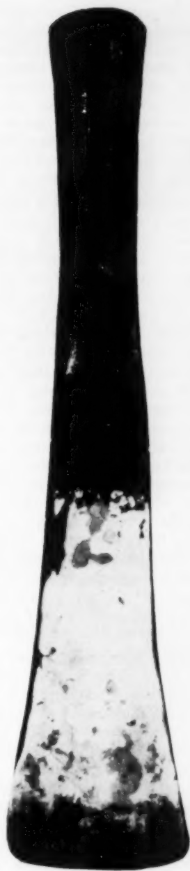
An implement known as a barretta, forged from a meteorite in the Village of Xiquipilco. For use, a handle is inserted in the sleeve at the top and the tool is used much as we use a crowbar.
